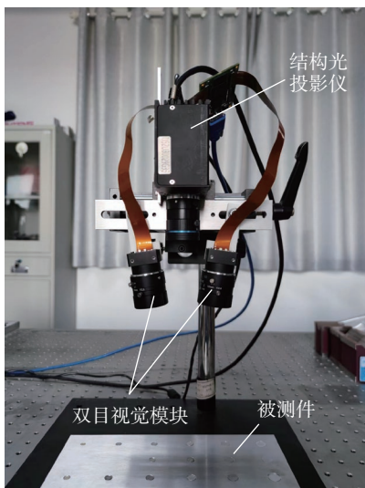
图1 基于结构光的双目视觉检测装置 Fig.1 Binocular vision inspection device based on structured light
